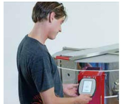
**ConeFire Mode** - Allows you to easily program the kiln based on the cone value and whether it is a bisque or glaze firing. Now it is faster than ever. An easy to edit screen lets you quickly change parameters from the last firing and start the program. You can also view the actual segments in the program and display a graph of the firing.
